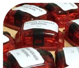
▲ Accelerometers (red devices)
